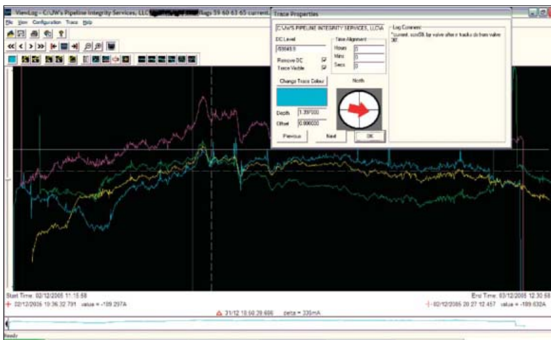
This computer display shows logged current measurement data at flags 59-65. Patterns can occur in smaller areas and the survey may not show all the patterns occurring between locations logged (Fig. 7).
